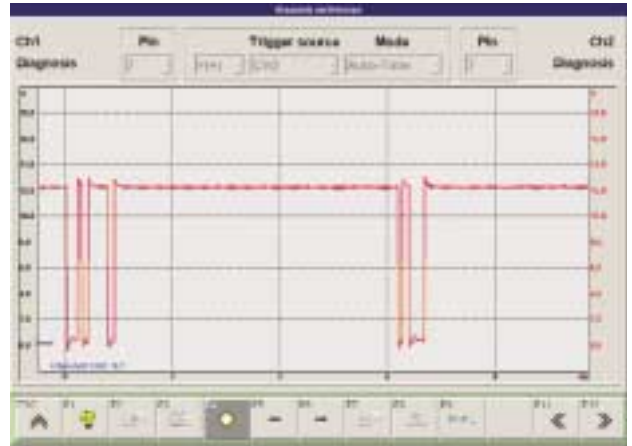
Improved error analysis with the diagnosis oscilloscope
