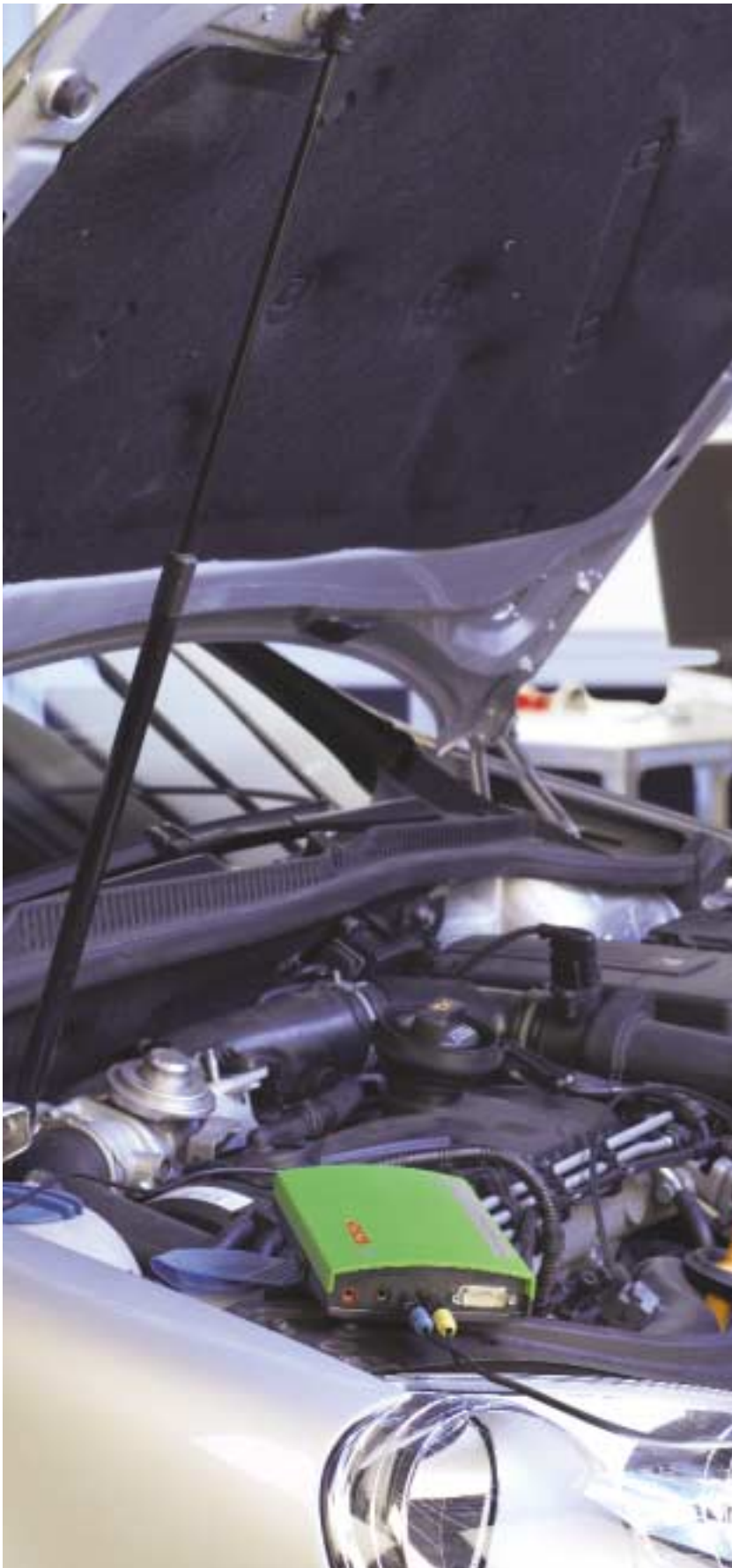
Control unit diagnosis in a workshop with radio technology up to 100 meters
