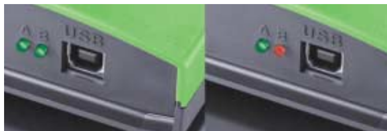
Status displays via LED on the KTS housing
